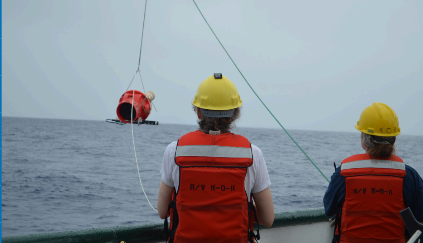
NOAA Affiliates Dr. Elizabeth Steffen (left) and Marine Tech Elizabeth Ricci (right) deploy a Deep Surrounding Oceanographic Lagrangian Observer (SOLO) Argo float from the R/V Ka'imikai-O-Kanaloa in 2018. The Deep SOLO float was developed by the Scripps Institute of Oceanography Instrument Development Group (SIO IDG), and this was the first Deep SOLO float to be deployed by NOAA Affiliates. (Image credit: NOAA)
