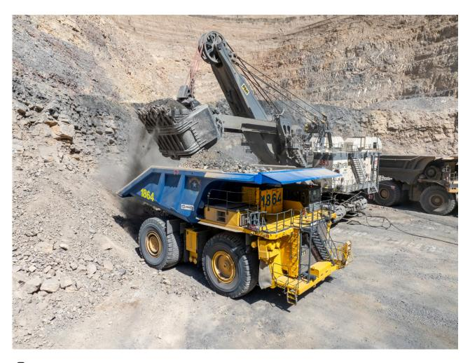
An electric shovel loading haul trucks at Nevada Gold Mines's open pit mining operations
