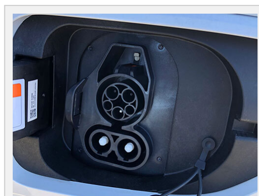
The Combined Charging System (CCS), also known as the SAE J1772 combo, charge port on a vehicle can be used to accept charge with Level 1, Level 2, or DC fast charging equipment.
