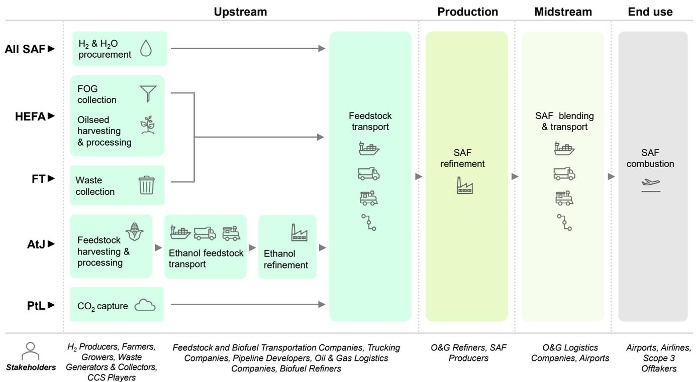
**Hydroprocessed Esters and Fatty Acids (HEFA)** requires triglyceride feedstocks such as oilseeds and waste fats, oils, and greases (FOGs). HEFA is the most mature technology pathway to produce SAF and is the only pathway that has been deployed at commercial scale.
