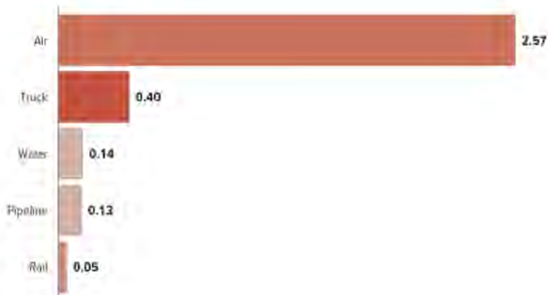
Average Carbon Dioxide Emissions per Ton-Mile of Freight, by Mode of Transportation, 2019 (CBO, 2022).
