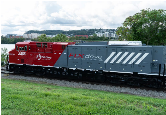
Figure 11: Wabtec 2.4 MWh FLXDrive battery locomotive 58
