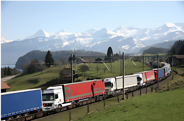
Figure 22: Roll-on/roll-off system in Switzerland. Image courtesy of Reservations Solutions Company (RALpin)
